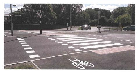
Figure 4- Example of a parallel crossing
